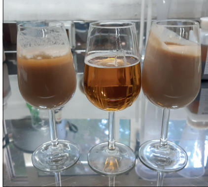
Inlet product, permeate, retentate after use of Omnia B filter
